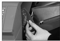
4. Set the blue separator shield lever to the **letter** required.
