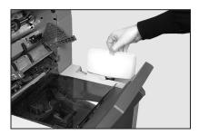
2. Open the envelope inverter access door and lift the insertion area plastic cover.
