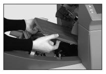
release them. Slide the plate into its location guides and release the catches to lock the plate in position.
