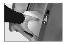
Press the envelope feeder loading switch again to raise the envelope stack to the normal feeding position.
