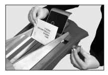
2. Refer to the labels located on the insert feeder. Match your insert type (slip, reply envelope, pre-folded or booklet) with the relevant icon and color indicator on each label.
