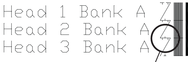
Head 3 is now correctly aligned
