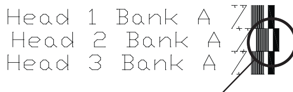
Head 2 misaligned horizontally
