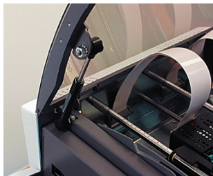
Properly installed shock
