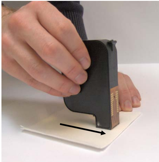
Figure 50: Cleaning the nozzle plate
